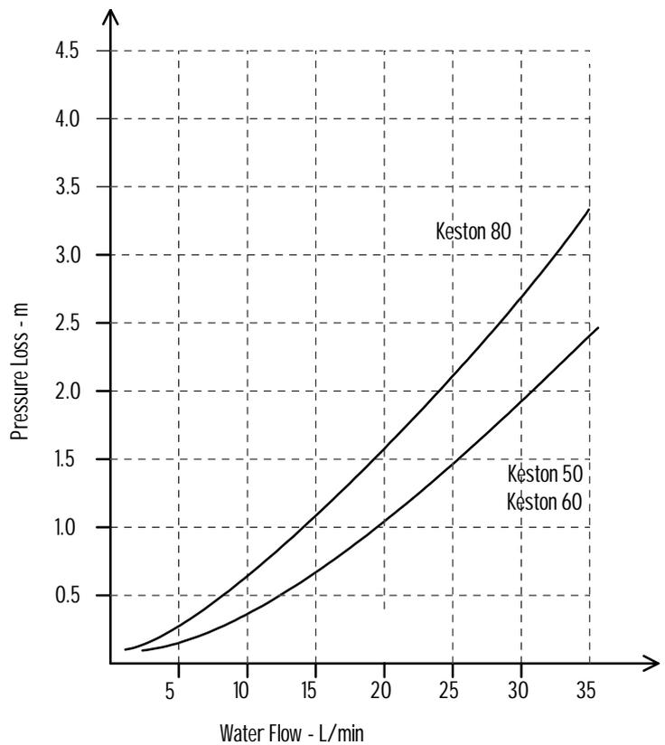
Figure 2.7.7 : Pressure Loss Graph
