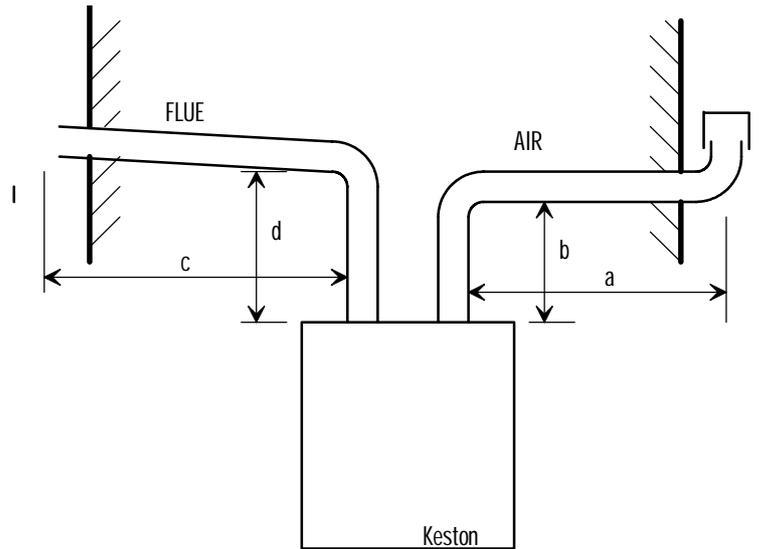
Figure 2.8.2 : Flue & Air Maximum Length Example
